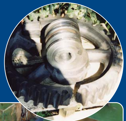
The original gearing proved to be badly damaged. New gears with improved ratios were manufactured and installed by Cast Iron Welding Services.
