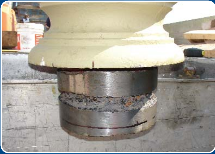
The column spigots were built up with gas fusion weld, and along with the mounting face, re-machined. The finished castings were then returned to site.
