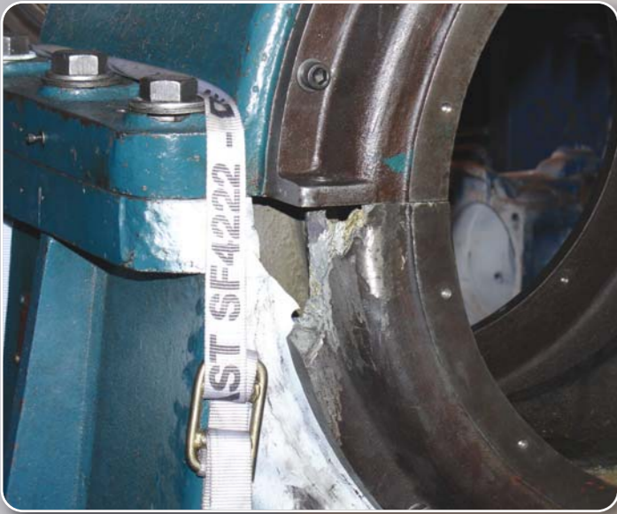
This component has a cracked flange. Once repaired the gas fusion weld will be virtually invisible.
