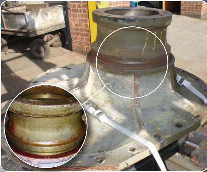
Military vehicle wheel support casting with worn boss. This was rebuilt and machined back to standard specification.
