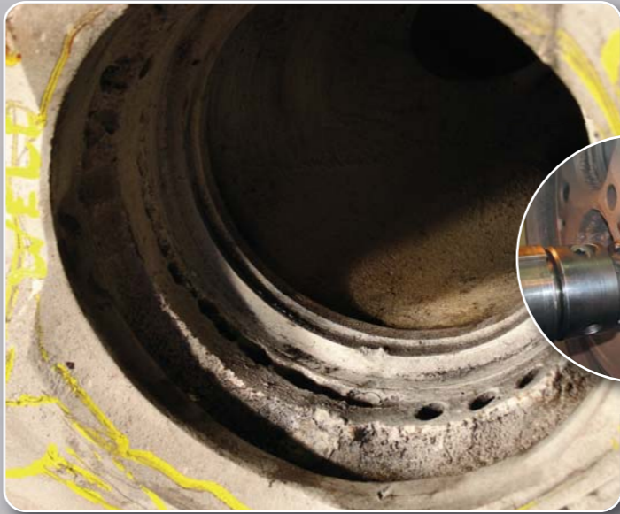
These eroded valve seat pockets will be gas fusion welded and will be machined to accept new valve seats.
