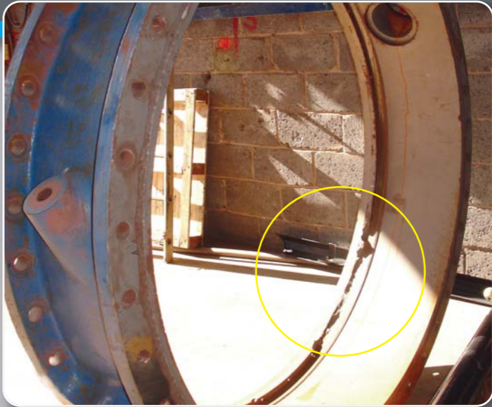
A valve body with eroded sections on the internals which will be built up and machined to standard size.
