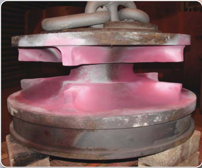
Ships chain winch with the locating dogs worn away, have been built up and ground to fit the locating dogs.
