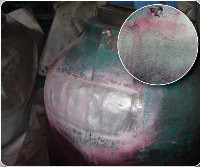
The finished repair having been crack and pressure tested.
