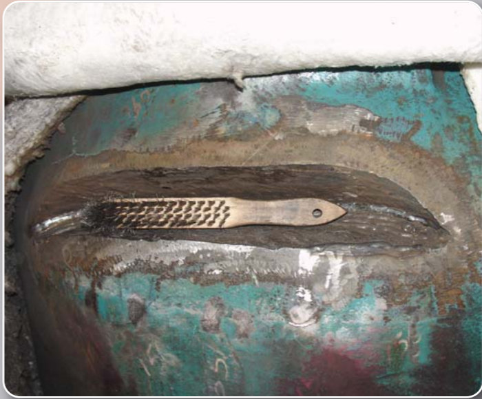
This cracked cylinder has been prepared for gas fusion welding.
