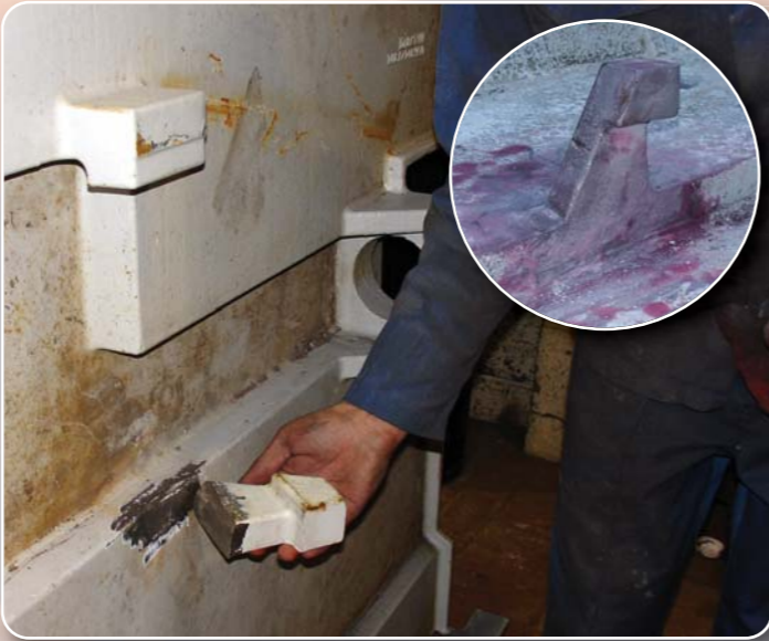
Machine bed with a broken lug. This will be gas fusion welded back into place.
