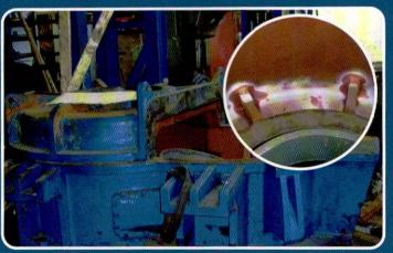
Gearbox with cracked internal webs which have been restored.
