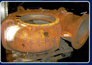
Due to the age of the component and the environment in to which it was to operate it was decided to further enhance the repair by the addition of strengthening ribs to the outer of the discharge channel.
