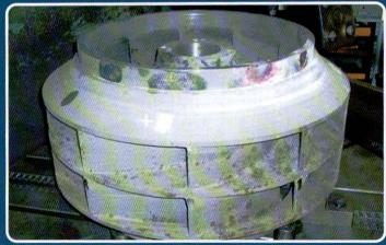
The blades of this impeller have been built up with gas fusion weld, then machined back to the original profile.
