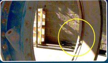
This butterfly valve had extensive erosion around its sealing areas. These were gas fusion welded ready for machining back to its original profile.
