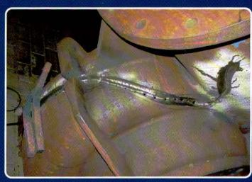
The component is then prepared for welding by removed the crack in it s entirety and to then establish a firm base of sound parent metal upon which to commence the welding process.
