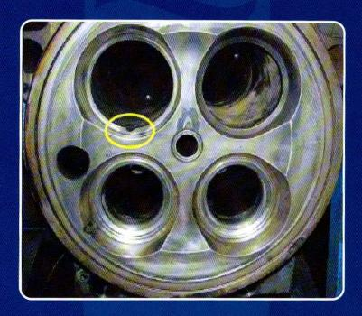
Burn-by damage to the exhaust cage seat landing.
