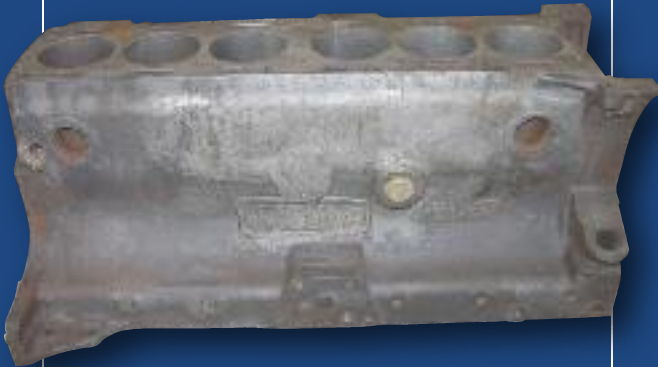
Jaguar 3.8 Litre block with water jacket corrosion damage.
