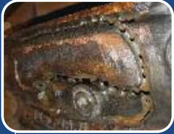
Jaguar 3.8 Litre block with water jacket corrosion damage.
