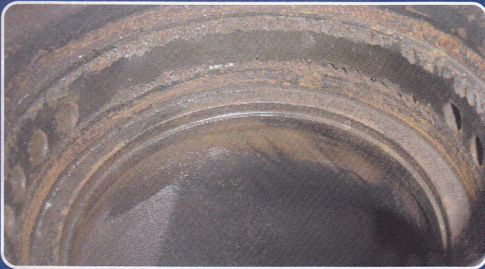
This picture shows eroded exhaust seat pockets having gone beyond the last standard oversize.
