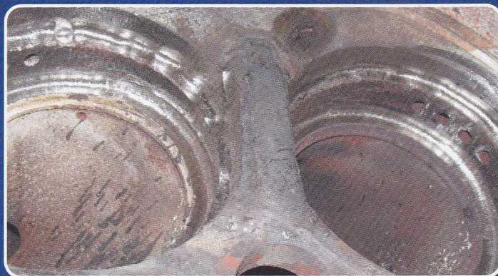
Weld repair stage 1: Repaired cross bore cooling channel.
